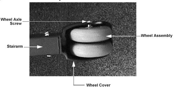
5. Install the replacement wheel assembly in the wheel cover. The replacement wheel axle screws that are supplied with the wheel assembly employ a loctite patch, no other locking means is required. If a wheel axle screw is being reused, apply a thin coat of blue loctite to the wheel axle screws. Install and hand tighten the two wheel axle screws. Torque the wheel cover screws to 25 in/lbs.
